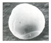
improve impact, nailing, stapling, and sanding properties of molded parts. The finest grades are used in RP/Composites including glass fiber reinforced products formed by both spray-up and hand lay-up production processes, where surface detail is critical. The coarser grades are used in cast or molded parts not requiring ultra-fine surface appearance.
